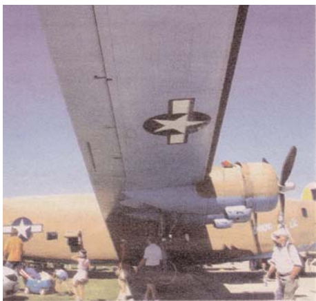
The 110-foot span of the Liberator Diamond 'Lil' is greater than that of a B-17. This wing incorporates the Davis high-lift airfoil and Fowler area-increasing flaps, new concepts on the cusp of World War II that helped give the Liberator its legendary long range and load-carrying capabilities.
